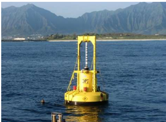
Wellengenerator Powerboy (Foto: Ocean Power Technologies)
